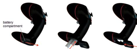
The charging port is at the bottom of the handle and has to be connected with the supplied battery charger. As soon as the charger is connected to Flystick2+ the charging process is started (red status LED: continuously active).
