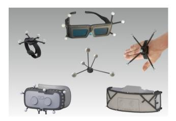
Targets consist of several markers (minimum 4), and provide 6DOF (degrees of freedom) data. We distinguish between **passive** and **active** types.
