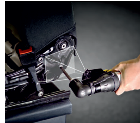
Recognition of various screw positions on a car seat with VERPOSE®
