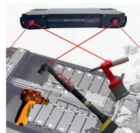
Identical and closely placed screw positions with EV battery connectors.
